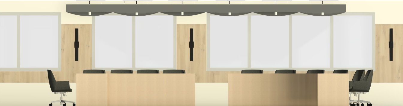
ACT Ceiling Grid and Tiles in Council Chamber with Linear Acoustic Baffles – Ebbs & Flows Pattern in smoke colour, Suspended over Millwork
